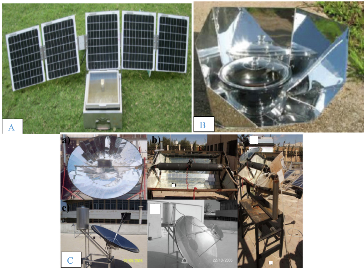
Fig. 2. Different types of SCs: (A) box SC (Joshi & Jani, 2015), (B) panel SC (Aramesh et al., 2019), (C) parabolic SC (Arunachala & Kundapur, 2020).
